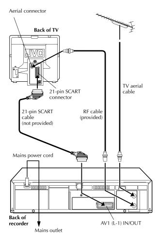
Make AV connection if your TV has a 21-pin AV input connector (SCART) in order to reduce the possibility of interference. And if you are using a stereo TV, you will need an optional 21-pin SCART cable in order to enjoy stereo playback of video tapes.
